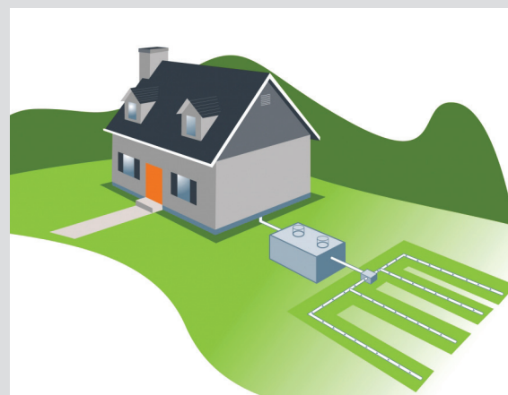
Diagram of a sample septic system.
